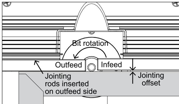
Use a scrap piece of wood to test the setup. If you feed the scrap past the bit and it runs into the leading end of the outfeed fence face, the fence is too far forward and you're not removing enough material. Use the micro-adjuster to move the fence back.
