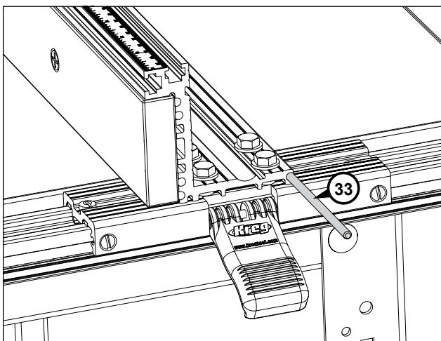
**9** To store the jointing rods (33), slide them into the round channel at the back edge of the fence extrusion base flange. (See **Jointing** under the section **Using Your Router Table Fence**.)
