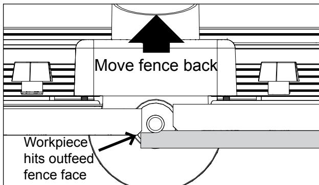
If the bit gouges the scrap at the trailing edge, the fence is too far back, and you're removing too much material. Use the micro-adjuster to move the fence forward.
